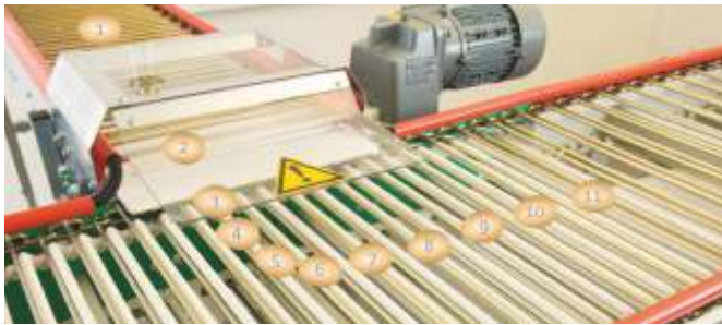
Conveyor chain with rods up/down (28°) Input unit chain
