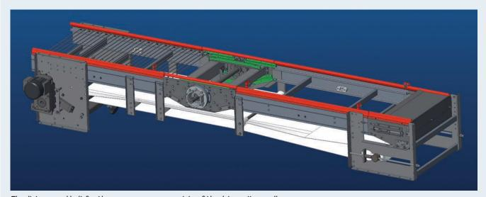
The dirt removal belt for the curve conveyor consists of the drive unit as well as the holders for the plastic fabric belt and the end unit. The belt speed of the dirt belt is 3.9 m /min.
